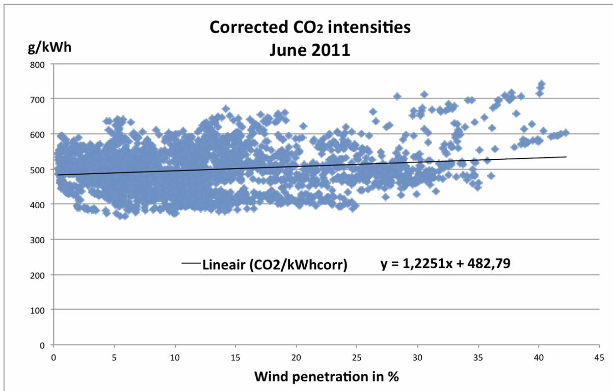
The next three Figures also show how when wind generation increases beyond a certain proportion of total supply, the level of CO2 emissions per MWh also start to rise again, because of the emissions from stand-by power stations that are not themselves generating power when in stand-by mode.
